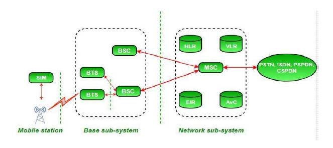
GSM stands for Global System for Mobile communication. Today, GSM is used by more than 800 million end users spread across 190 countries which represent around 70 percent of today's digital wireless market. GSM is combination of TDMA (Time Division Multiple Access), FDMA (Frequency Division Multiple Access) and Frequency hopping.
